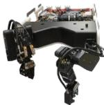
Dual five-function heavy duty manipulator system. Manipulator camera options available
