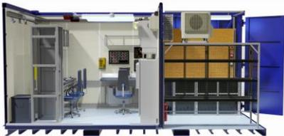
Safe Area 20ft split Control Cabin with a Pilot Control section and a separate high voltage PSU section. Fitted with electric power distribution panels, lighting, air conditioning, heating, 19 inch racks and escape hatch is available as is a Zone II upgrade.
